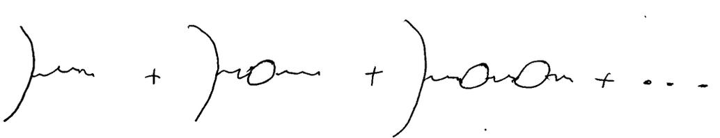
Fig 1. *Modification of the Coulomb potential due to the dressing of the photon propagator.*
