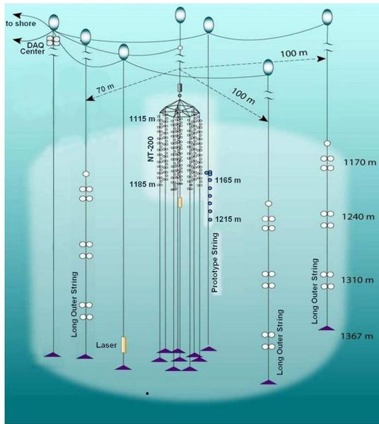
Figure 1: The Baikal Telescope NT200+ as of 2008: the compact NT200 (center), 3 long outer strings and the new technology km3-prototype string.
