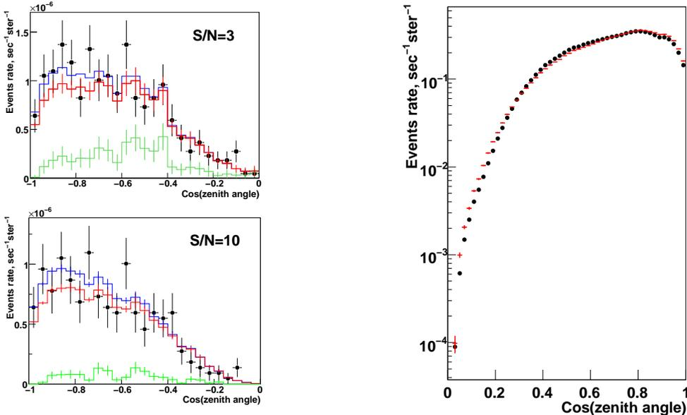
Figure 3: Distribution of  $\cos(\text{zenith})$  for muon events. Left: neutrino event samples (data - symbols, MC - histograms (from top): sig+bkg for non-osc., oscillation and bkg); Right: downward atmospheric muons (data - symbols, MC - histogram).
