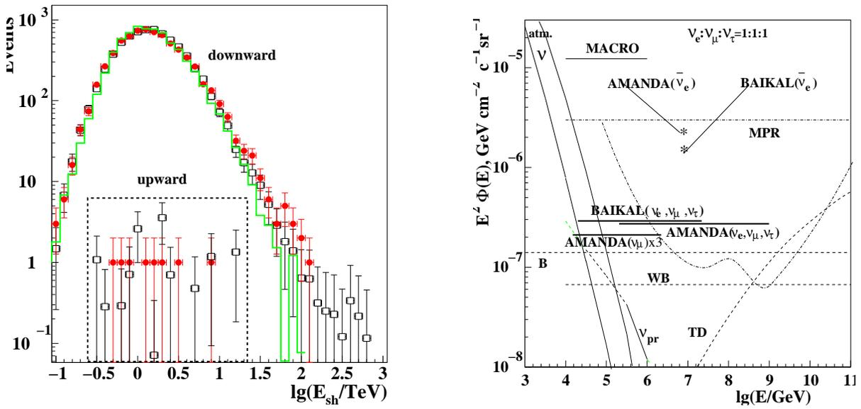
Figure 6: Left panel: Reconstructed cascade energy distribution for data (red dots) and for MC-generated atmospheric muons (boxes); true MC energy distribution given as histogram. Right panel: All-flavor neutrino flux bounds and predictions in different models of neutrino sources compared to experimental upper limits to  $E^{-2}$  fluxes obtained by this analysis and other experiments (see text).
