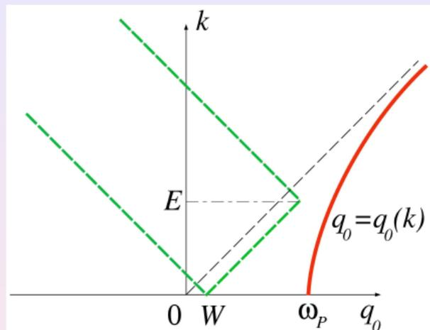
For the process  $\nu_L \rightarrow \nu_R \gamma^*$  to be possible, the neutrino energy must exceed a **threshold** value:
