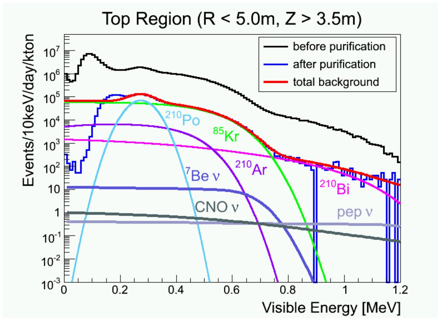
About  $1700\text{m}^3$  of the KamLAND scintillator were purified last year. Due to mixing between purified and non-purified scintillator purification effect is smaller than needed for the  $^7\text{Be}$  observation. The upper part of the detector is filled with scintillator after a 2<sup>nd</sup> pass through the system. The 2<sup>nd</sup> purification campaign started 2 weeks ago and will continue for 6 months.
