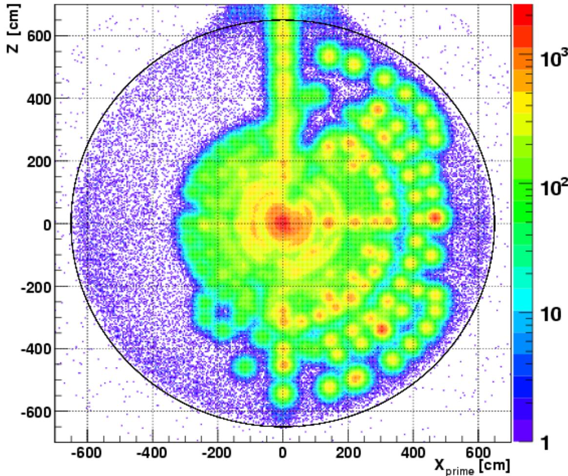
Off-axis calibration system was used to deploy  $^{241}\text{Am}^9\text{Be}$ ,  $^{210}\text{Po}^{13}\text{C}$ ,  $^{60}\text{C}$ ,  $^{68}\text{Ge}$ , and  $^{203}\text{Hg}$  sources into KamLAND and study vertex reconstruction biases at distances up to 5.5m away from the detector center. We found that the event **vertex fitter** reconstructs event's position with a **bias < 3cm** within the 5.5m volume which corresponds to **1.6%** systematic error.
