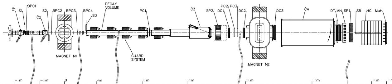
Figure 1: Elevation view of the "ISTRA+" detector.
