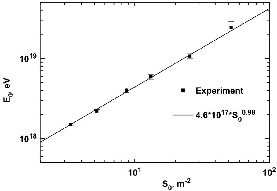
Figure 1: Relation between shower energy  $E_0$  and parameter  $S_0$  determined by the calorimetric method at Yakutsk array. The line corresponds to equation (1).
