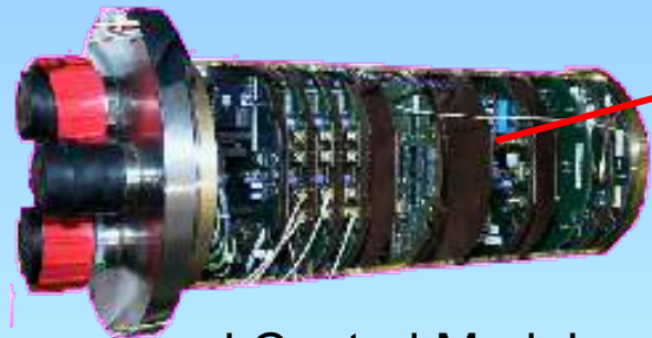
Local Control Module (in Ti Cylinder): DAQ and Slow Control + Compass Cards
