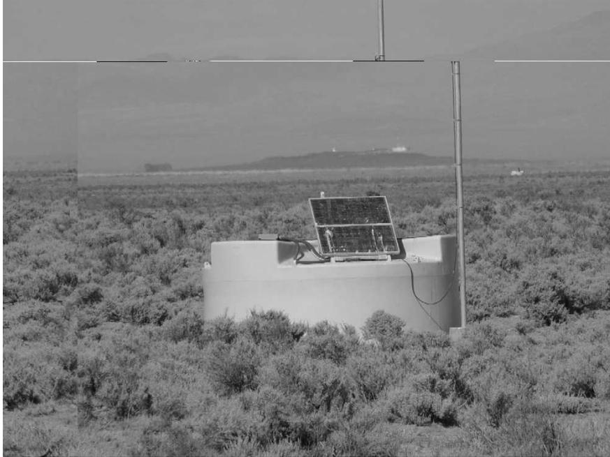
Figure 3: One of the 1600 water Cherenkov detectors (the surface array), spaced by  $1.5\text{ km}$  over area of  $3000\text{ km}^2$ . The solar panel and the communication antenna is seen. At the horizon a fluorescence detector on a hill can be seen.
