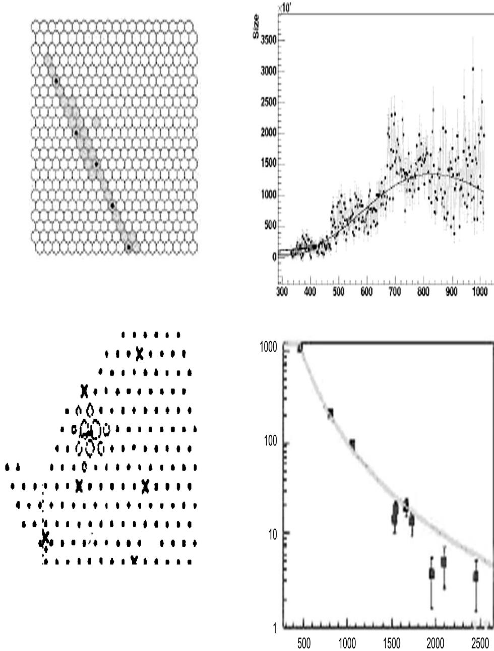
Figure 6: A hybrid shower, ie. registered by both types of detectors. In the upper right panel - reconstructed number of particles has to be multiplied by  $10^7$ . See text.
